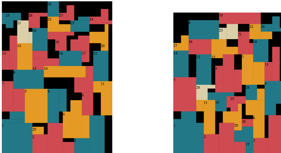
Figure 3: An example when the best-fit algorithm performs better (left: the bottom-left algorithm, right: the best-fit algorithm)
